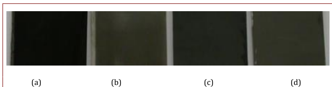
Figure 5. Thick films of enamels prepared with (a) commercial copper-chromite pigment, (b) BP600, (c) BP900 and (d) BP1100 heat-treated at 700 °C for 5 min
